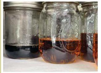
On the left is oil treated with other bleaching clays. On the right is the same oil treated with W3.
